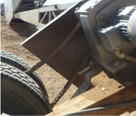
Drive chain resting without tension.
