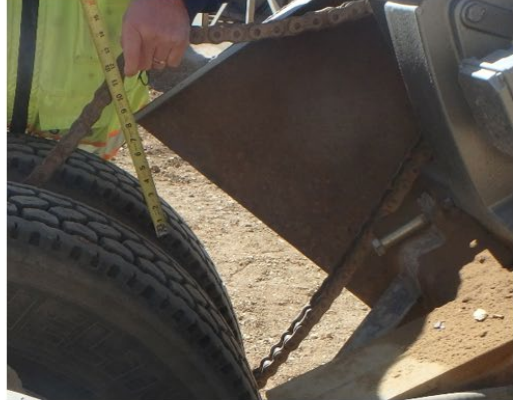
Drive chain slack approximately 14 inches.
