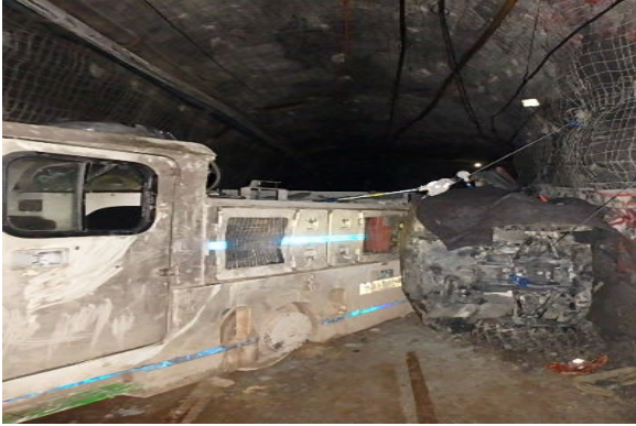
Two miners traveling in a personnel carrier collided with a locomotive traveling in the opposite direction.
