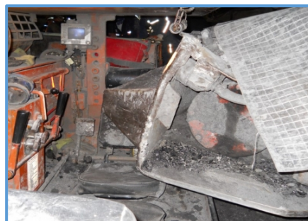
A miner died when underground shuttle cars collided in an intersection. One shuttle car trammed through a ventilation curtain without stopping or warning.
