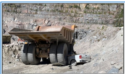
Roadway design and poor visibility at a nearly blind intersection were the root causes of a miner's death when his pickup was crushed by a haul truck.
