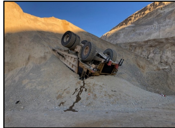
The edge of the dump bank failed, causing the haul truck to travel backwards and overturn, landing on the roof of the cab.
