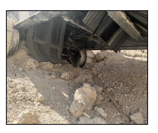
A 62 year-old mechanic was cleaning underneath a portable crusher when he became entangled in a belt conveyor. The mechanic entered the small area below the portable crusher without locking and tagging out.
