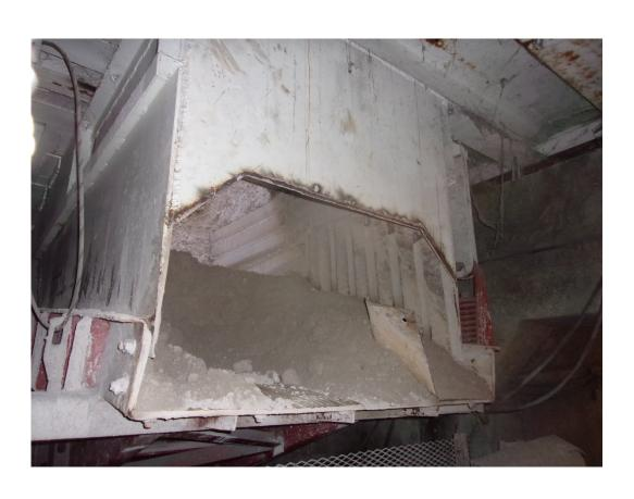
A 39 year-old maintenance lead person entered a pan feeder to remove a piece of angle iron. The angle iron prevented a gate, that was in a chute, from closing. Material from a surge pile above the chute fell through the open gate, into the pan feeder, and engulfed him.
