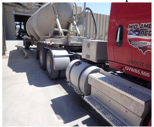
A contract truck driver was attempting to close the hatch on top of his trailer when he fell approximately ten feet to the ground. The driver was not wearing fall protection. The driver was admitted to the hospital with broken ribs and other injuries.
