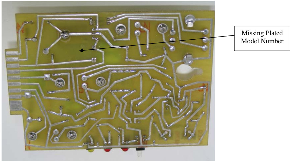
Figure 4 - Non-conforming Circuit Board Trace Side (Bottom)
