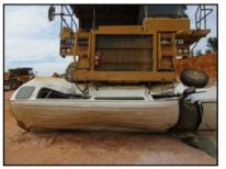
Large Vehicles Hitting Small Vehicles Surface mining vehicles can be several stories tall and are capable of destroying smaller vehicles that cannot be seen by the operator. Traffic controls, training, and avoiding distractions are key to enhancing safety. Collision warning and avoidance systems can also help.
