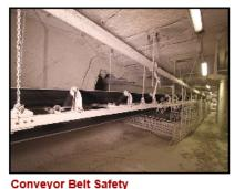
Conveyor belts and their components pose serious risks to miners working on or around them. It's important to install adequate guarding to prevent contact, provide and use crossovers and cross unders, and lock out energy sources and block motion whenever performing maintenance.
