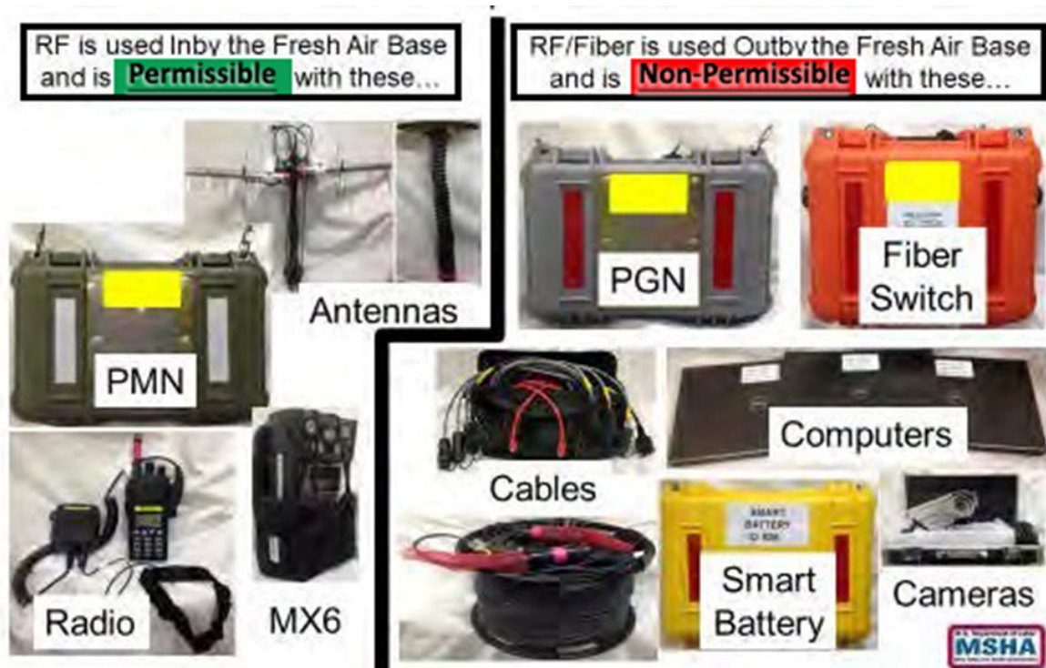
Visual 9: Underground Communication System Components
