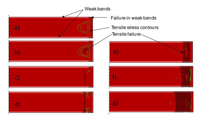
**Figure 18.** Stages of failure development in a beam of strong rock encased between two weak bands.
