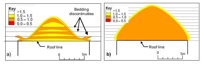
Figure 37. Vertical cross section through a heading showing rock failure index values (a) with three 1-m thick (3.3 ft) bedding discontinuities in the roof and (b) thinly laminated roof.
