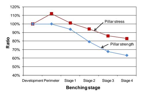
**Figure 23.** Change in the average vertical pillar stress and pillar strength relative to development during various stages of bench mining, for a pillar with a width-to-height ratio of 1.5 based on the results of numerical models.
