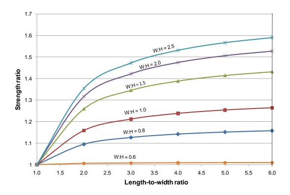
**Figure 24.** Strength increase caused by increasing pillar length for pillars with various width-to-height ratios. Results from calibrated numerical models assuming rock failure initiates as spalling followed by shearing.
