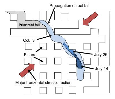
Figure 34. Plan view showing the development of a stress-related roof fall in the direction perpendicular to the direction of the major horizontal stress [lannacchione et al. 2003].
