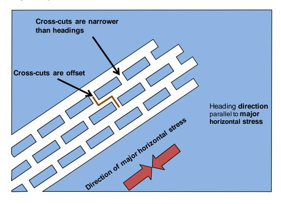
**Figure 38.** Diagram showing room-and-pillar layout modified to minimize the potential impact of horizontal, stress-related damage.
