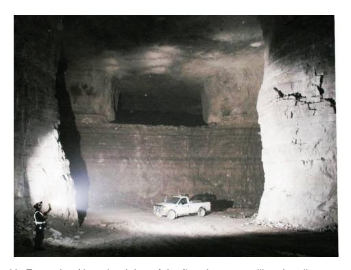
Figure 19. Example of bench mining of the floor between pillars in a limestone mine.
