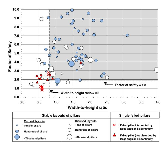
**Figure 25.** Chart showing the factor of safety against width-to-height ratio using equation 7. Current and disused pillar layouts are shown as well as single failed pillars. The recommended area for pillar design is shaded.
