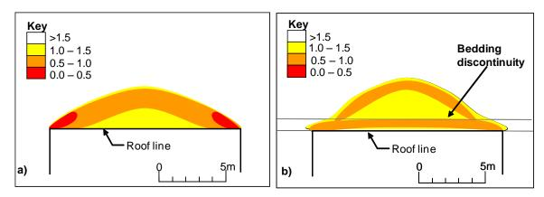
Figure 36. Vertical cross section through a heading showing rock failure index values (a) without bedding discontinuities and (b) with a bedding discontinuity 1 m (3.3 ft) above the roofline.
