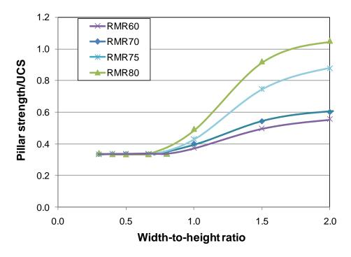
**Figure 11.** Effect of width-to-height ratio and rock mass rating (RMR) on pillar strength, based on numerical model results.
