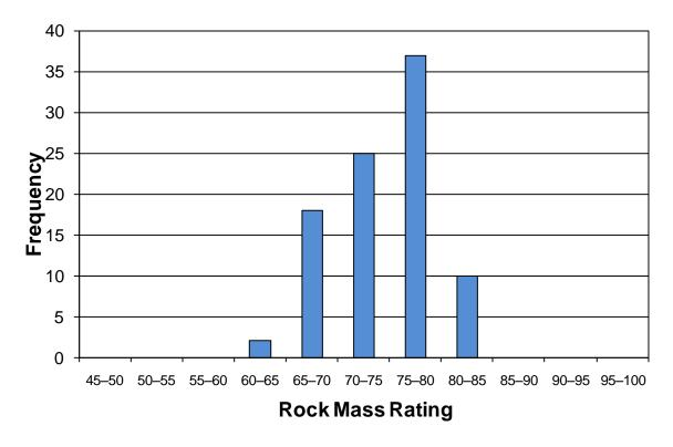
**Figure 2.** Distribution of rock mass rating (RMR) values in stone mines obtained by direct classification of rock exposure in underground stone mines and laboratory testing of rock cores.
