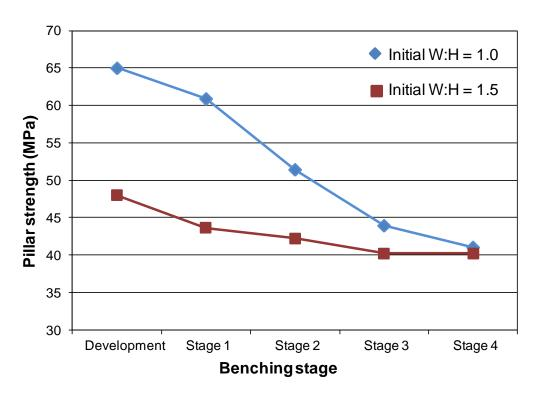
**Figure 21.** Results of numerical modeling showing strength reduction of pillars with initial width-to-height ratios of 1.0 and 1.5 from initial development through various stages of bench mining. Final width-to-height ratios at Stage 4 are 0.5 and 0.75.
