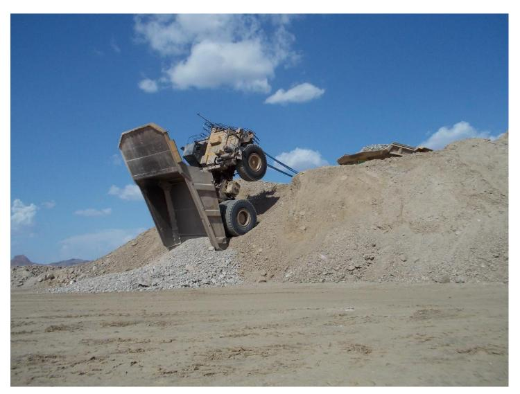
7/25/2021 – Dump site – Roll-over accident – The outer edge of the dump site gave way, causing the truck to tip over.
