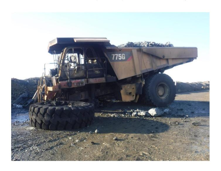
10/25/2021 — Fire — Non-Injury — Right rear brake overheated on the haul truck resulting in a fire.
