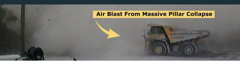
Since October 2020, four massive pillar collapses have occurred in limestone mines. Each was accompanied by a powerful airblast and the formation of a large surface sinkhole. Fortunately they did not result in any injuries. In 2015, three miners were seriously injured by an airblast from a fifth pillar collapse.
