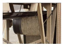
This photo shows buildup on a bend pulley. In 2024 a miner lost a thumb when he removed a guard and began to clean a rotating bend pulley with a 15-inch-long pry bar.
