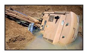
Operating equipment near a body of water can pose a potential hazard in your job. Several miners have died in drowning or drowning-related accidents.
