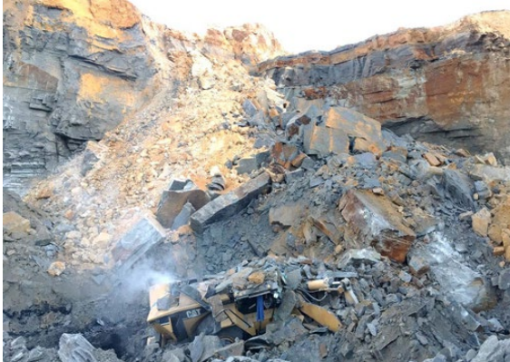
A miner was fatally injured at a surface coal mine while operating a front-end loader to remove shot rock near the base of a 63 ft. highwall.
