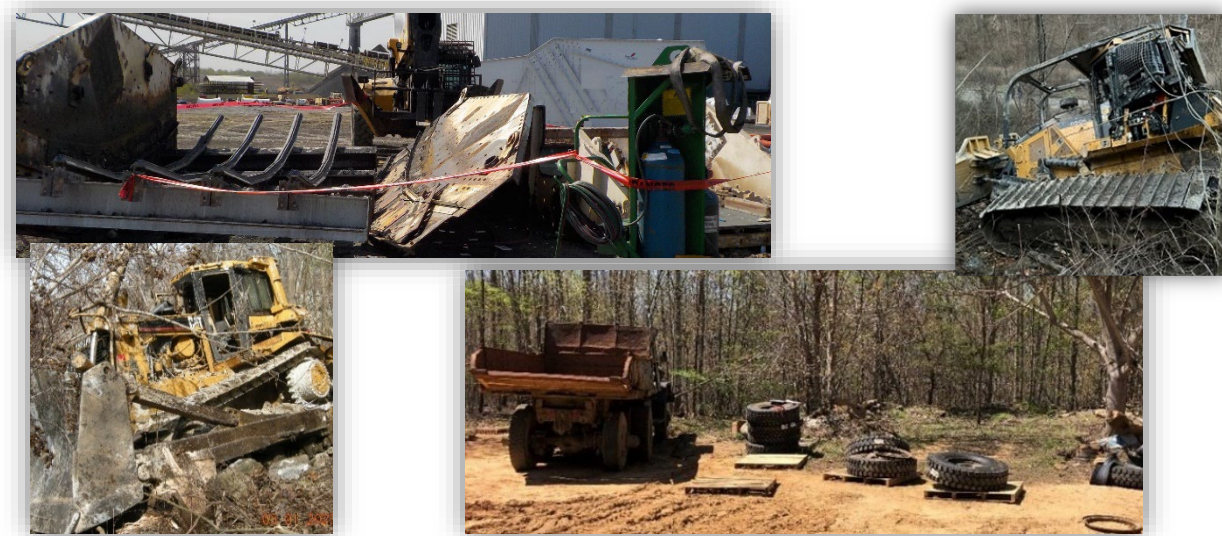
(Left to Right) Shaker screen disassembly. Bulldozer rolled down an embankment. Locking Ring dislodged from truck wheel. Bulldozer rolled down an embankment.
