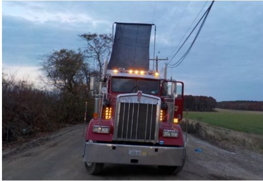
A truck driver was electrocuted when he tried to re-enter the truck's cab while the trailer's tarping mechanism was in contact with an energized overhead high-voltage power line.
