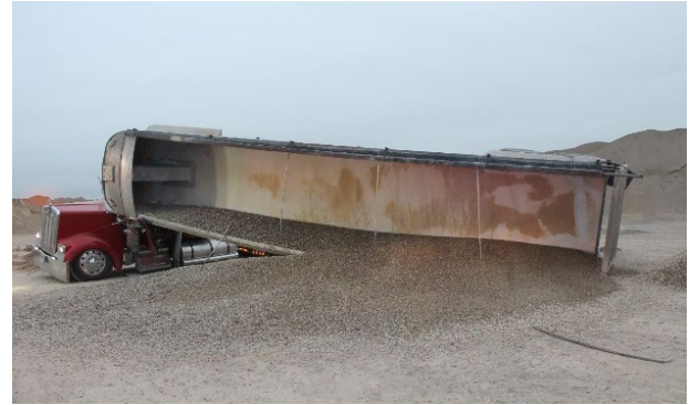
A truck driver died when his trailer tipped over onto the cab of the tractor. The driver was dumping part of the load of gravel from the trailer.
