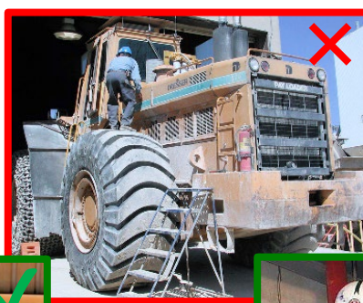
Left: Unsafe - Mechanic with no fall protection
