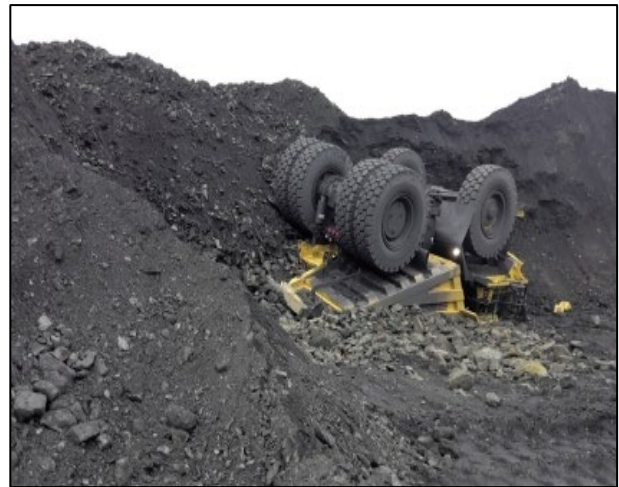
A miner was fatally injured when their haul truck traveled over the edge of a stockpile at the dump point and overturned.
