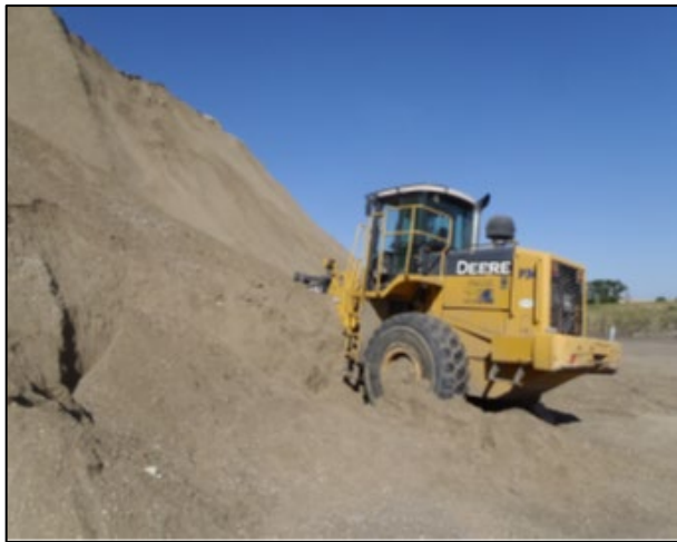
A miner was fatally injured while working near the toe of a stockpile. Upon exiting the front-end loader, the operator was engulfed by the unstable stockpile.
