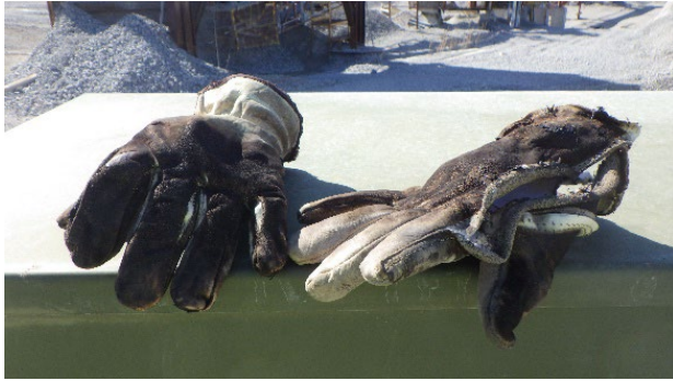
An electrician received burns from an arc flash when he cut an energized power line.
