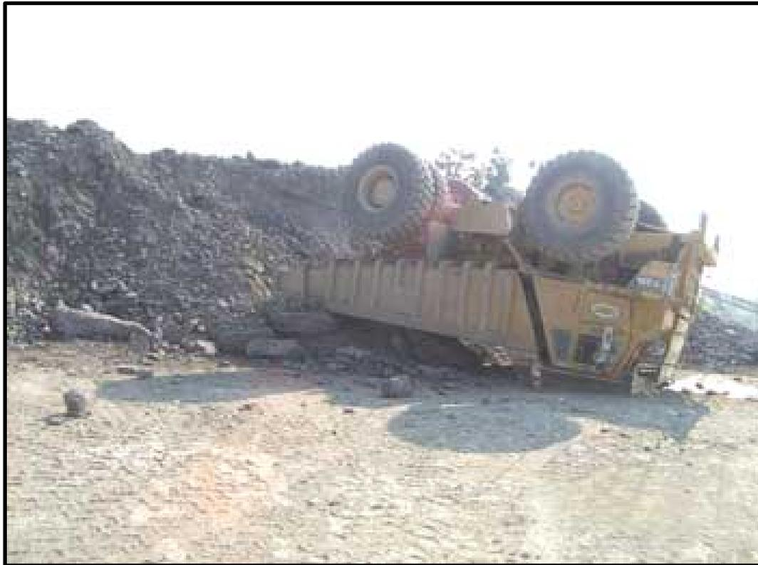
On September 13, 2005, a 64-year old truck driver, with 25 years mining experience, was fatally injured at a crushed stone operation. The victim, who was not wearing his seatbelt, was dumping material over a 20-foot high stockpile when the truck overturned..
