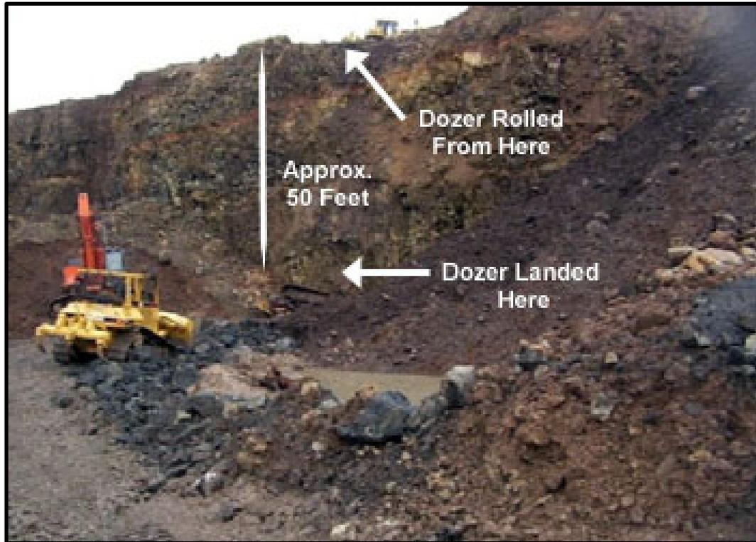
On January 27, 2006, a 60-year old heavy equipment operator with 10 years mining experience was fatally injured at a crushed stone operation. He was operating a dozer to prepare a bench for drilling. The dozer traveled over the edge of a 50-foot highwall and fell to the quarry floor, submerging the cab in several feet of mud and water.
