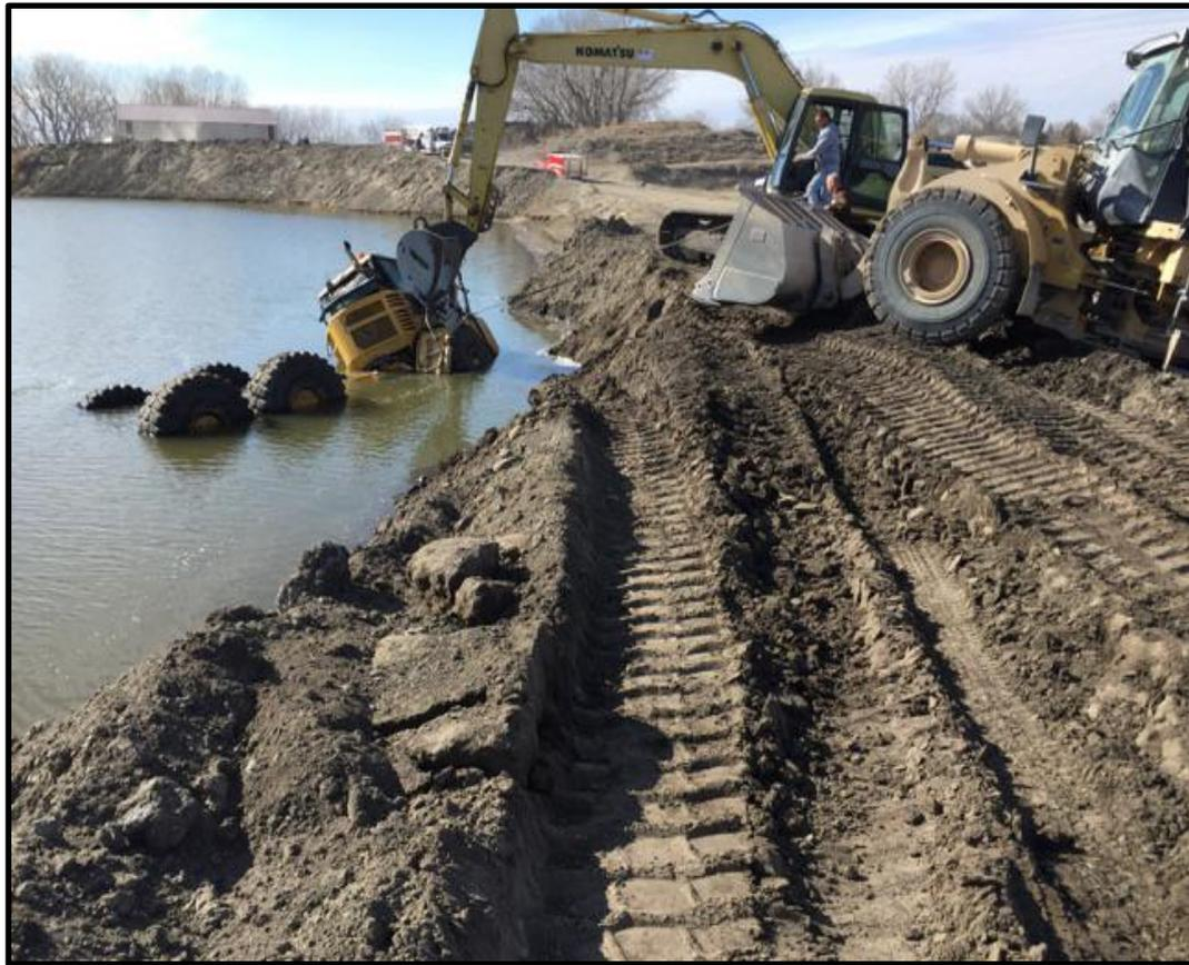
On March 17, 2015, a 44-year old haul truck driver with 4 days of experience was injured at a dredge operation. He was operating a loaded articulated haul truck along an elevated roadway next to a dredge pond. After traveling about 125 yards from the loading point, the haul truck drifted into the water. The victim was removed from the truck, transported to a hospital, and then transferred to a trauma center where he died on March 19, 2015
