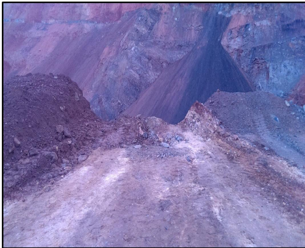
On March 8, 2016, a 54-year old miner with 5 years of mining experience was killed at a surface sand and gravel operation. The miner backed his haul truck over a dump site and the driver was found at the bottom of the embankment, 60 feet below. The victim was found unresponsive and partially submerged in water. CPR was attempted, but the victim was not able to be resuscitated.
