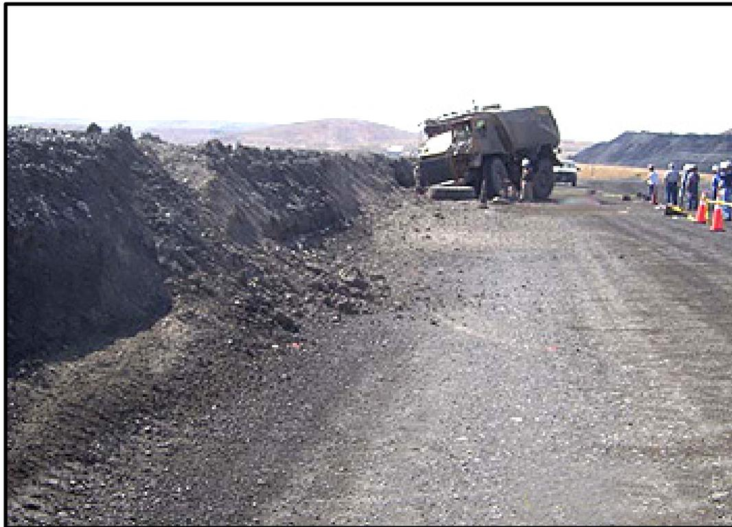
On July 30, 2005, a 23-year old contractor equipment operator, with 20 months mining experience, was fatally injured at a surface gold mine. The victim was operating a water truck that left the roadway and climbed the berm, causing it to overturn and land back on the haul road. The victim, who was not wearing a seat belt, was ejected from the cab of the truck.
