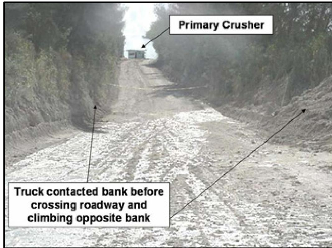
On August 13, 2005, a 56-year old haul truck driver, with 12 days mining experience, was fatally injured at a crushed stone operation. The victim was operating a haul truck from the primary crusher to the pit. As the truck descended the haul road into the pit, it struck the bank, traveled across the road, climbed the berm, and entered a water filled pit.
