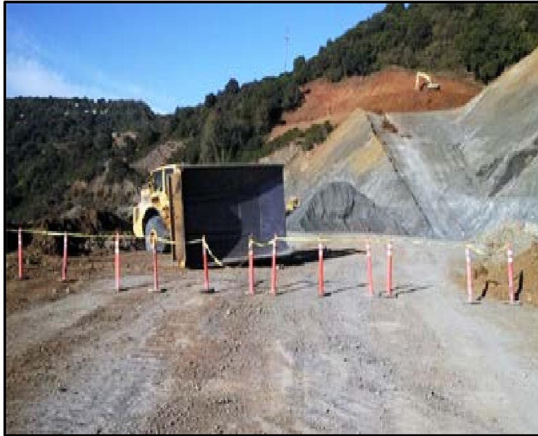
On June 13, 2013, a 50-year old mechanic with 15 years of experience was killed at a stone operation. He was operating a 35 ton articulated haul truck down a haul road. The truck went out of control and hit a berm, propelling it in the air. The truck came to a stop with the bed overturned and the cab upright. The victim was ejected from the truck.
