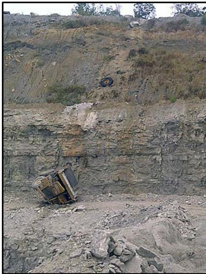
On September 16, 2013, a 58-year old truck driver with 25 years of experience was killed at a crushed stone operation. The victim was driving a loaded haul truck out of a quarry when the truck traveled through a berm and over an 80-foot highwall. The victim was ejected from the truck.
