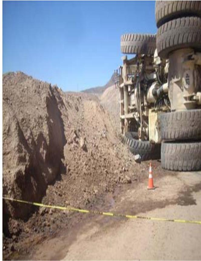
On September 27, 2009, a 28 year-old truck driver with 2 years of experience was fatally injured at a copper operation. He was operating a 240-ton haul truck that left the haul road and climbed a berm, causing it to overturn and land on the haul road. The victim, who was not wearing a seat belt, fell from the cab of the truck.
