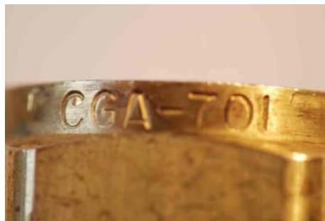
CGA designation on high pressure fitting (nut)
