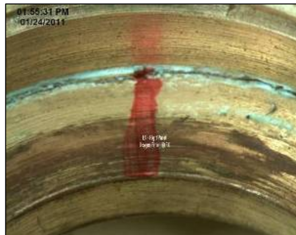
Figure 2 – magnified view inside brass fitting showing cracking (this fitting was still intact and held compressed gas)
