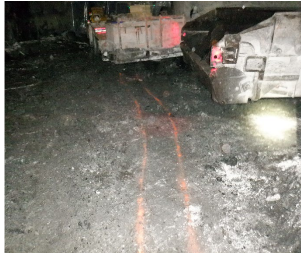
A miner was severely injured when he was pinned between a ram car and the coal rib.
