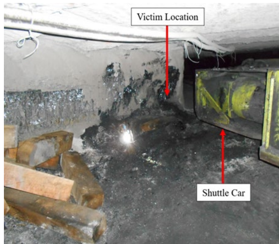
A miner died after he was pinned between a shuttle car and a coal rib.
