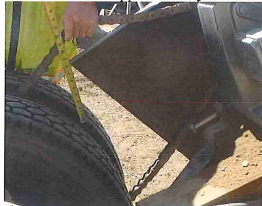
Drive chain slack approximately 14 inches.
