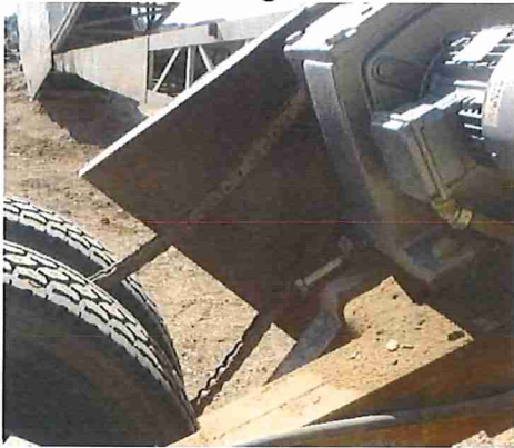
Drive chain resting without tension.
