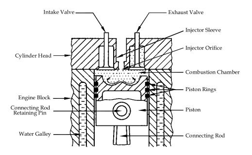
**SKETCH 2** Typical sketch showing injector removed
