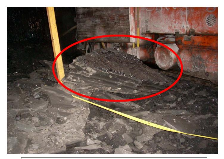
Rock that struck victim was triangular in shape and measured approximately 4.5 feet by 3.1 feet by 3.5 feet, and ranged from 9 inches to 11.5 inches thick.
