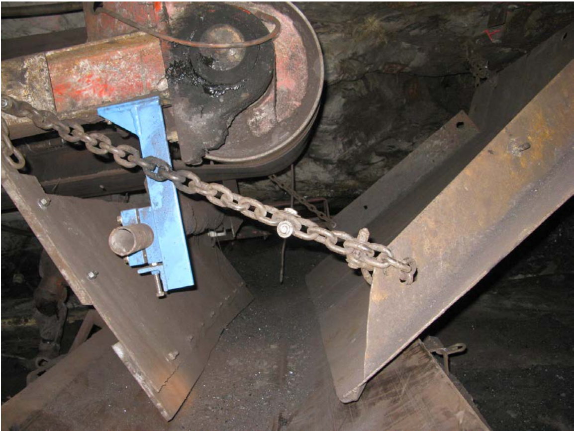
Photo of Reconstructed Accident Scene – Minus Discharge Roller Guarding
