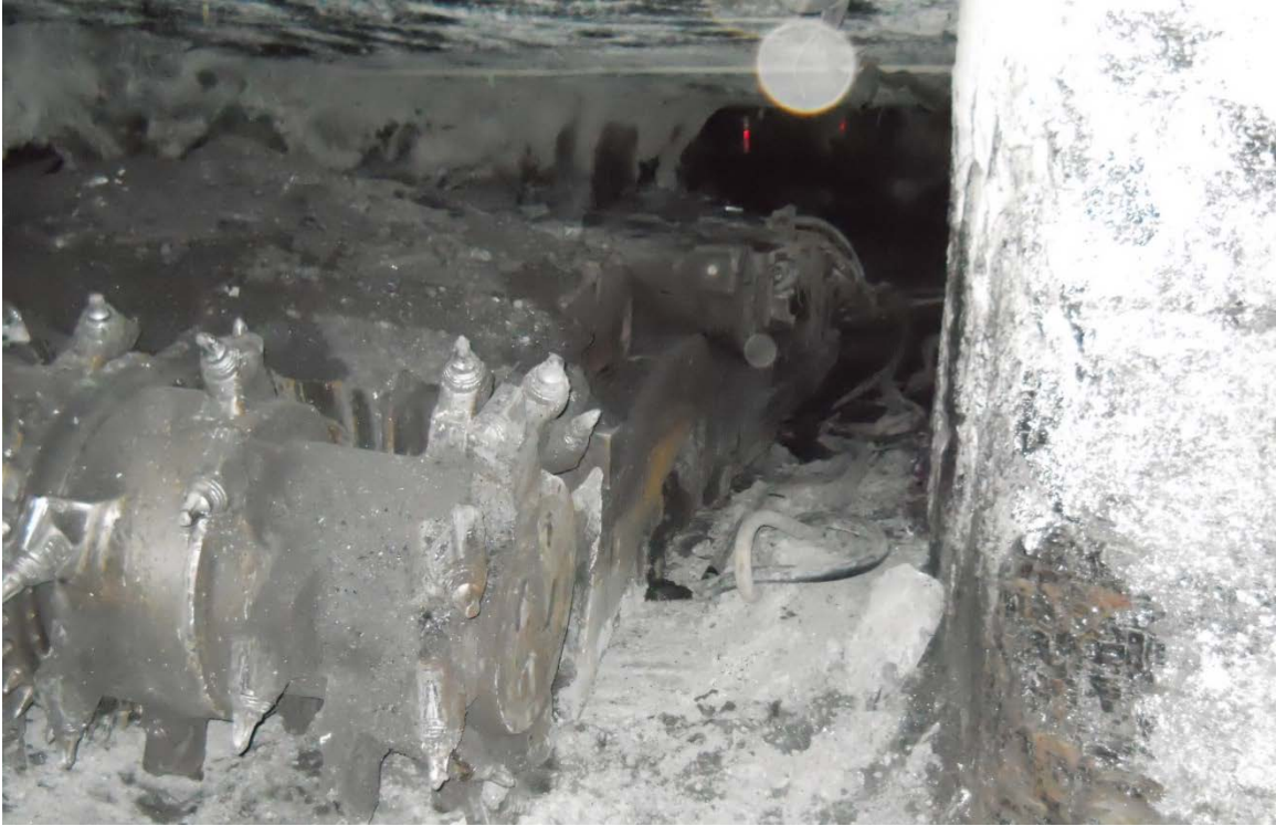
Photograph Of Accident Scene Showing Continuous Mining Machine And Coal Rib
