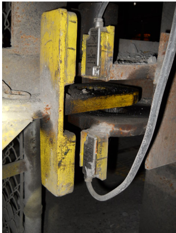
New Safety Switch Actuators Required by MSHA (post accident) Installed with Tamper Proof Bolts
