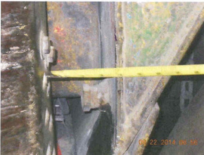
Wagner frame to frame closure as measured at 3 1/2 inches.
