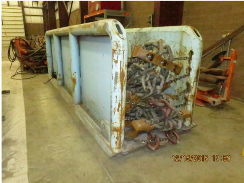
Photo 3: Oblique View of a Loaded Chain Tub with Conveyor Chain Showing General Arrangement
