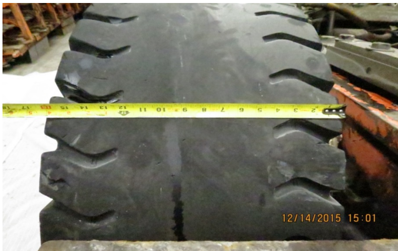
Photo 4: View of Tractor's Left Rear Tire Showing Tread Condition
