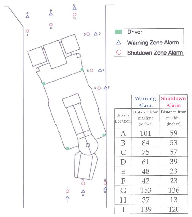
Note: Location (H) is measured from the end of the tail. Locations (G) and (I) are measured from the rear of the machine.
