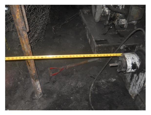
This photo shows the space that existed between the guard and the roller at the time of the accident. It also shows the stud bolts extending from the inby tandem roller shaft. These bolts are similar to the bolts that extended from the outby roller shaft where the accident occurred.
