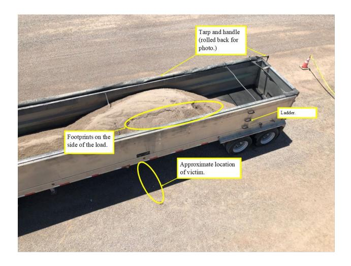
Appendix D Photo showing the end-dump trailer ladder, the tarp and tarp crank handle
