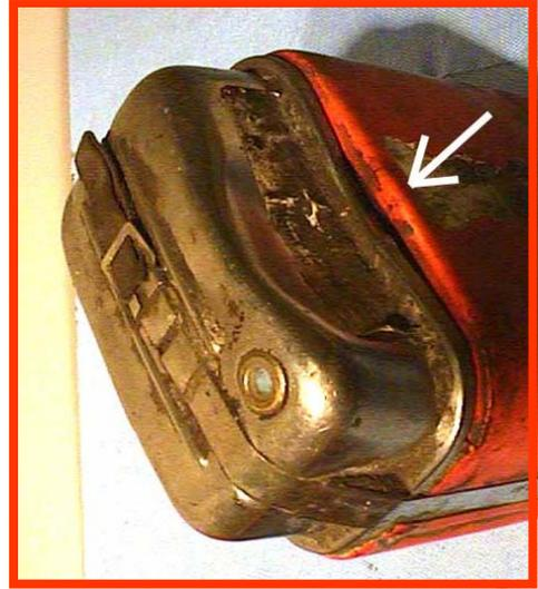
This unit has received a severe impact to its top cover. As a result, the top cover has a significant dent and the seal ring has been displaced.
