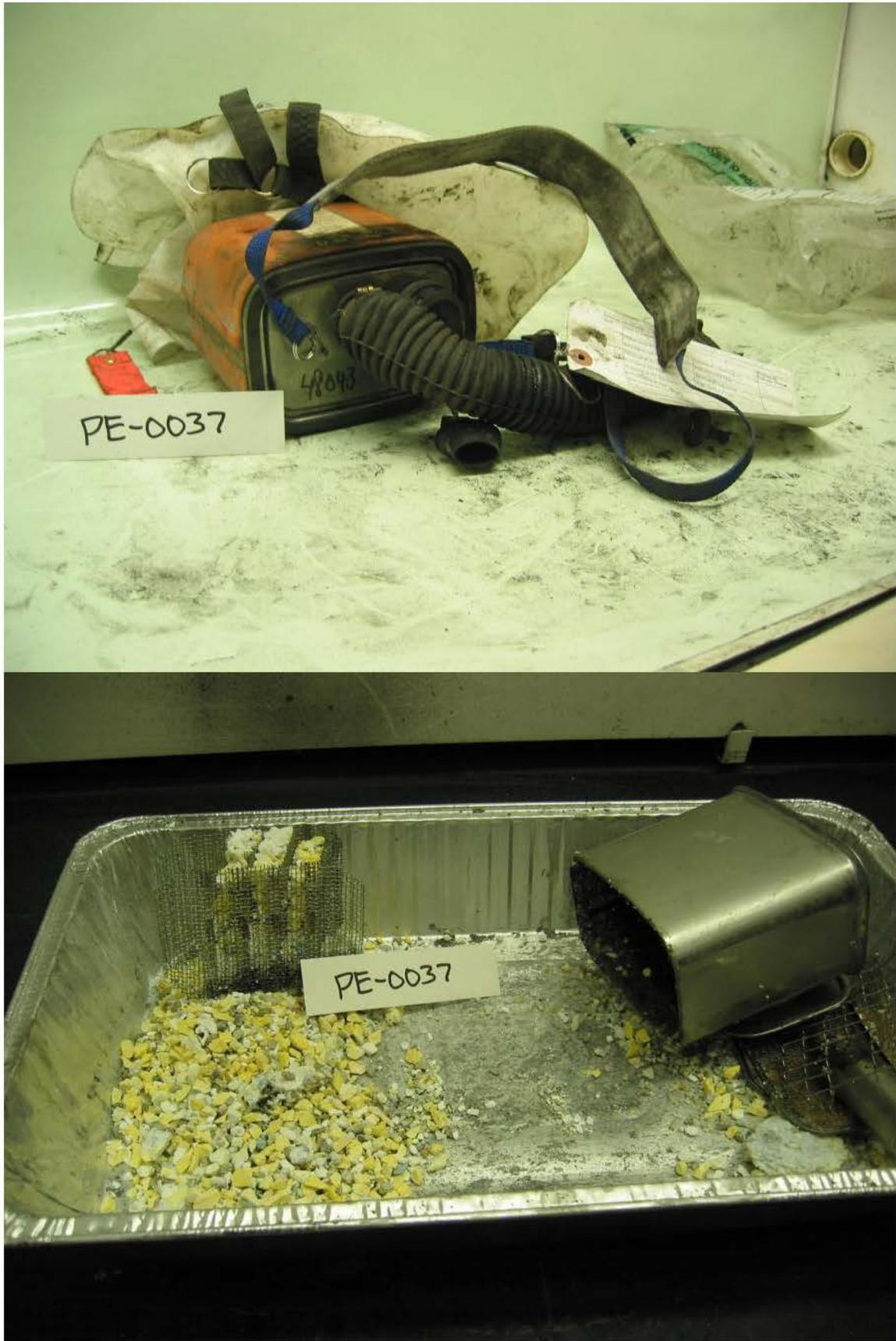
Figure 16 - Unit PE-0037, as Received and Remaining Chemical
