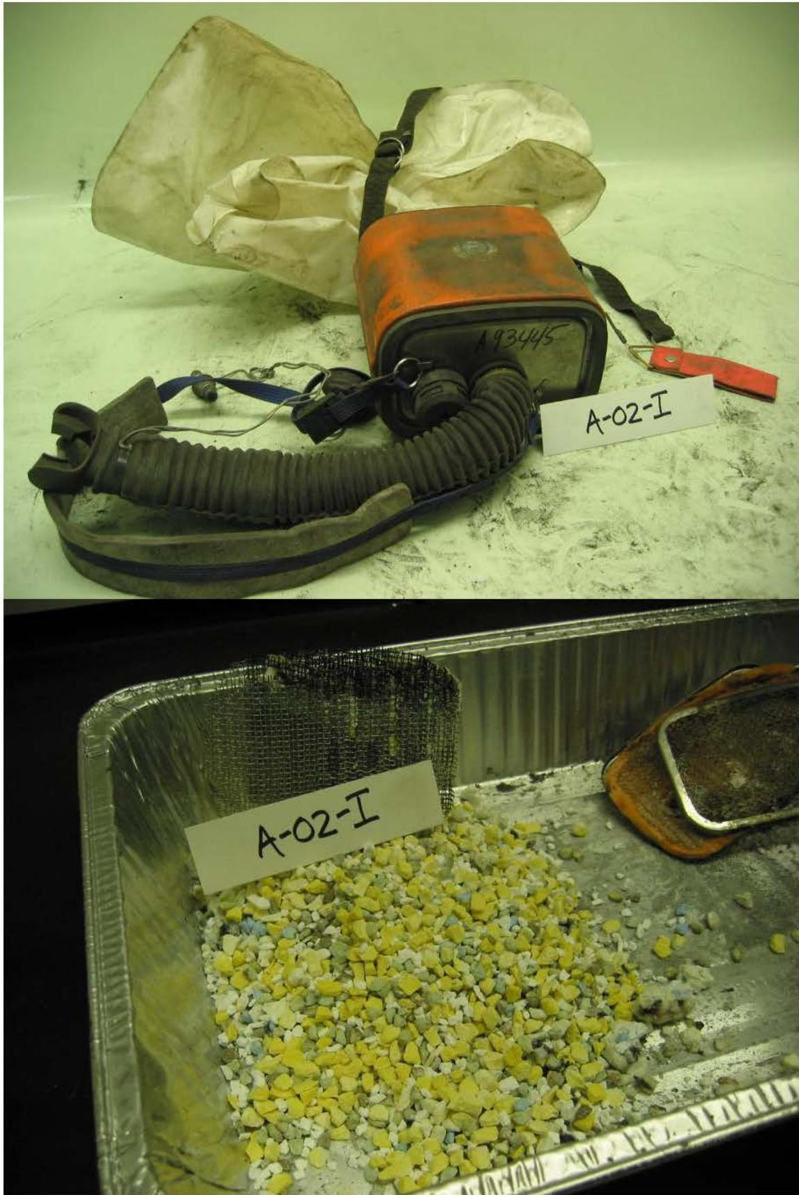
Figure 14 - Unit A-02-I, as Received and Remaining Chemical
