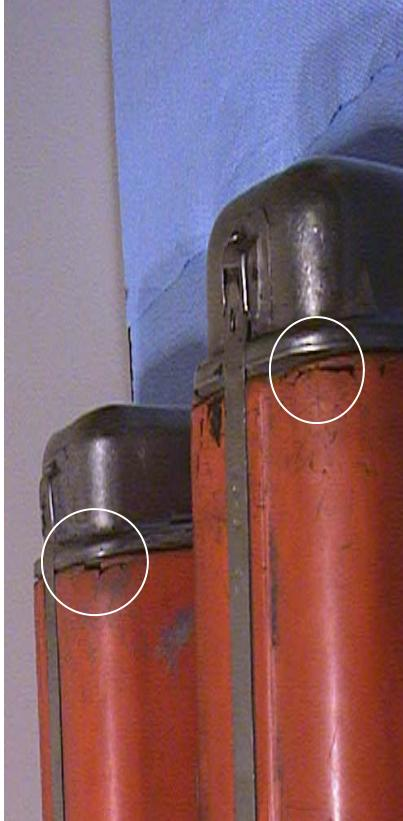
These wear points are the result of abrasion and minor impacts that do not adversely affect the SR-100 performance. These units may remain in service if they pass the remainder of inspection criteria.
