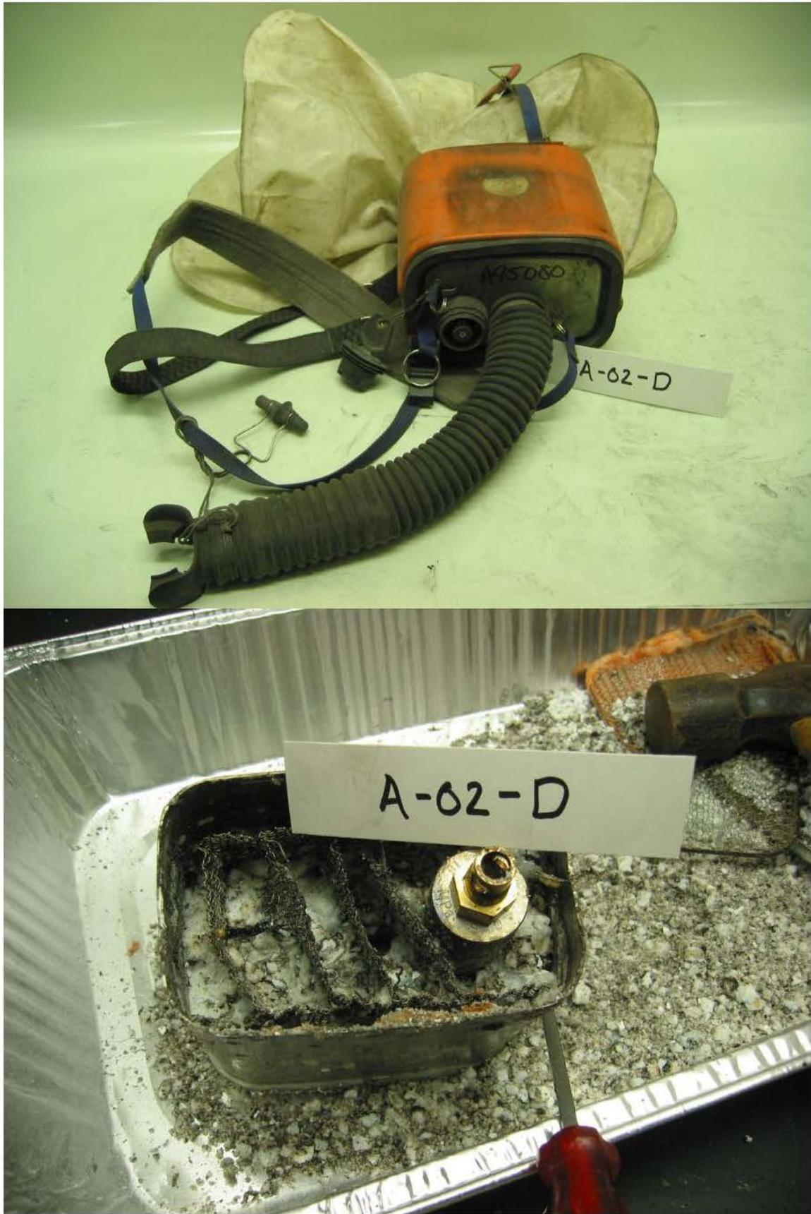
Figure 9 - Unit A-02-D, as Received and Remaining Chemical
