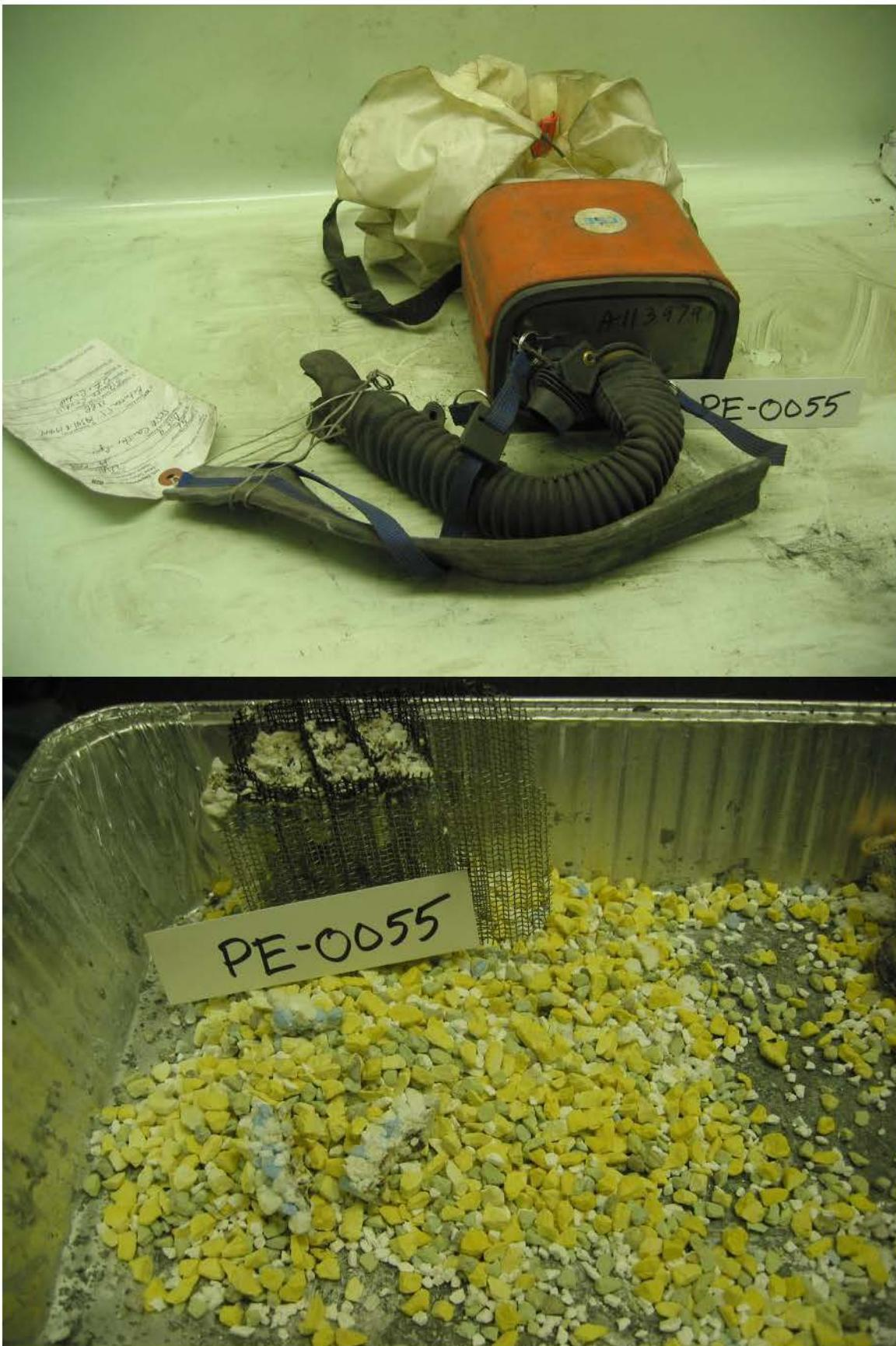
Figure 20 - Unit PE-0055, as Received and Remaining Chemical
