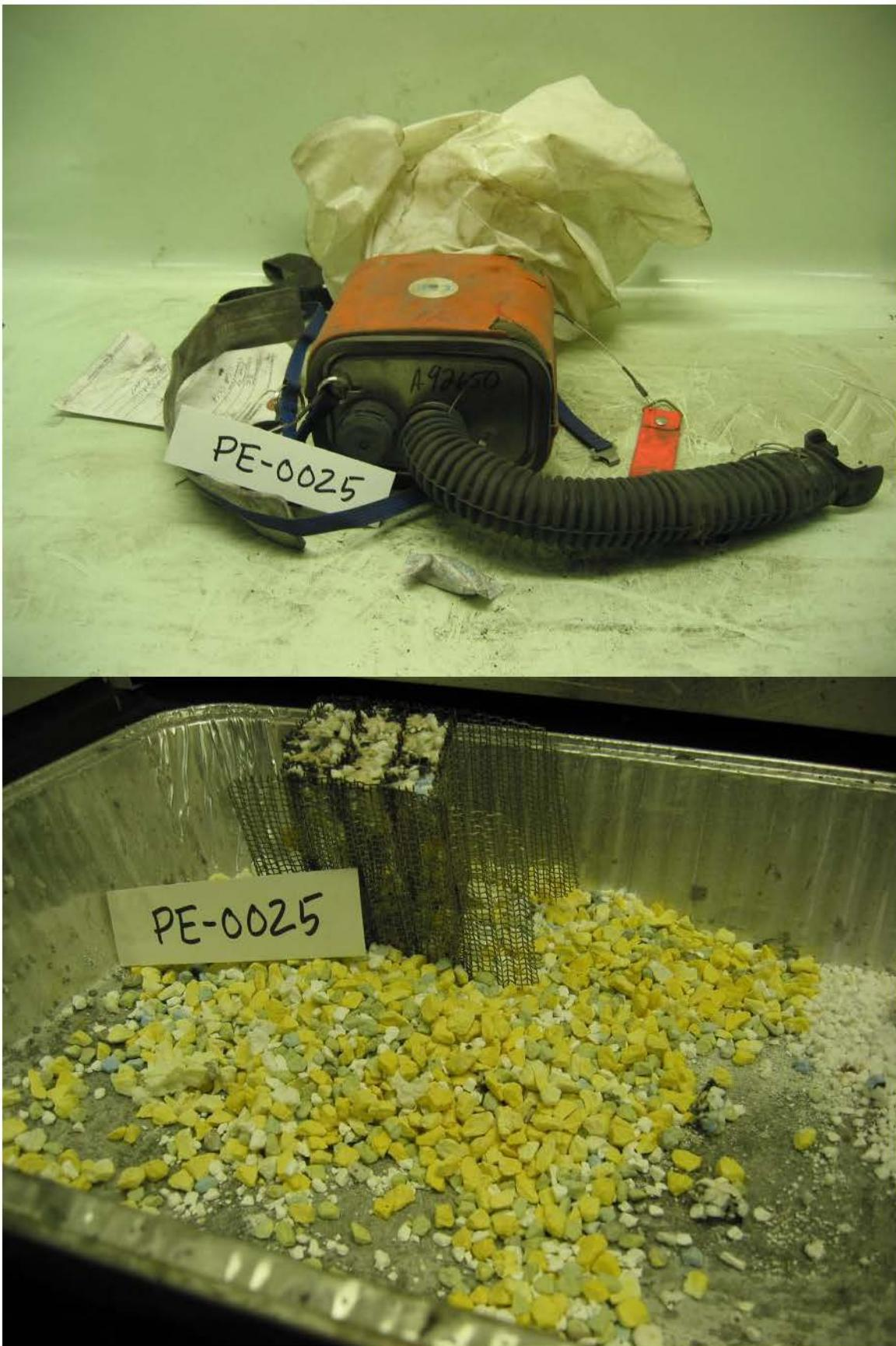
Figure 21 - Unit PE-0025, as Received and Remaining Chemical
