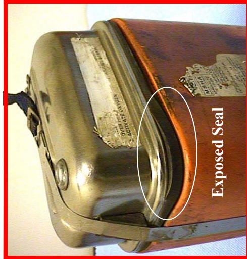
This unit fails the visual inspection because its seal has been displaced and is protruding from under the stainless steel cover.
