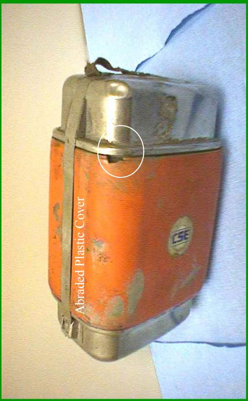
This unit's condition shows normal wear and tear. The abraded corner on the plastic cover and minor dent in the stainless steel top cover do not cause the unit to fail visual inspection. The unit may remain in service if it passes the remainder of the inspection.
