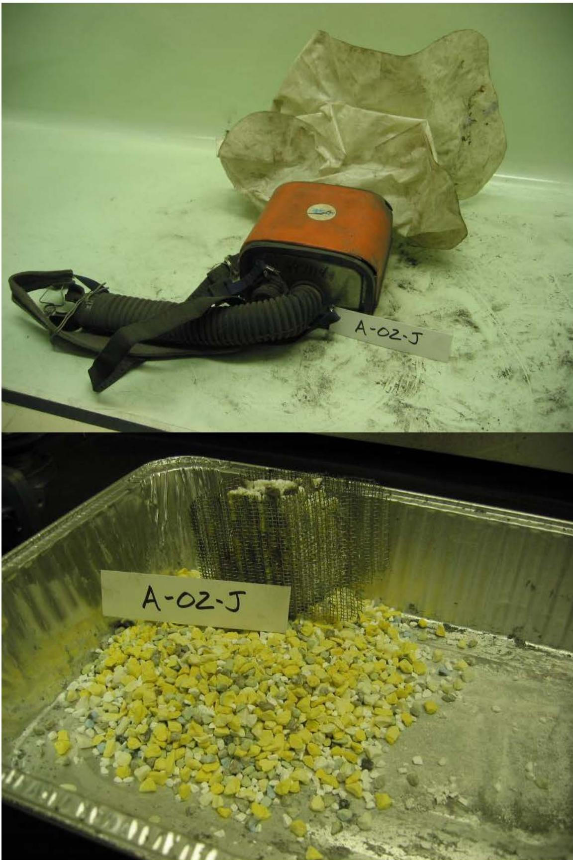
Figure 15 - Unit A-02-J, as Received and Remaining Chemical
