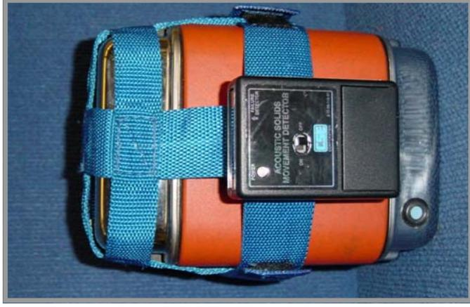
Acoustic Solids Movement Detector Mounted on a SR-100
