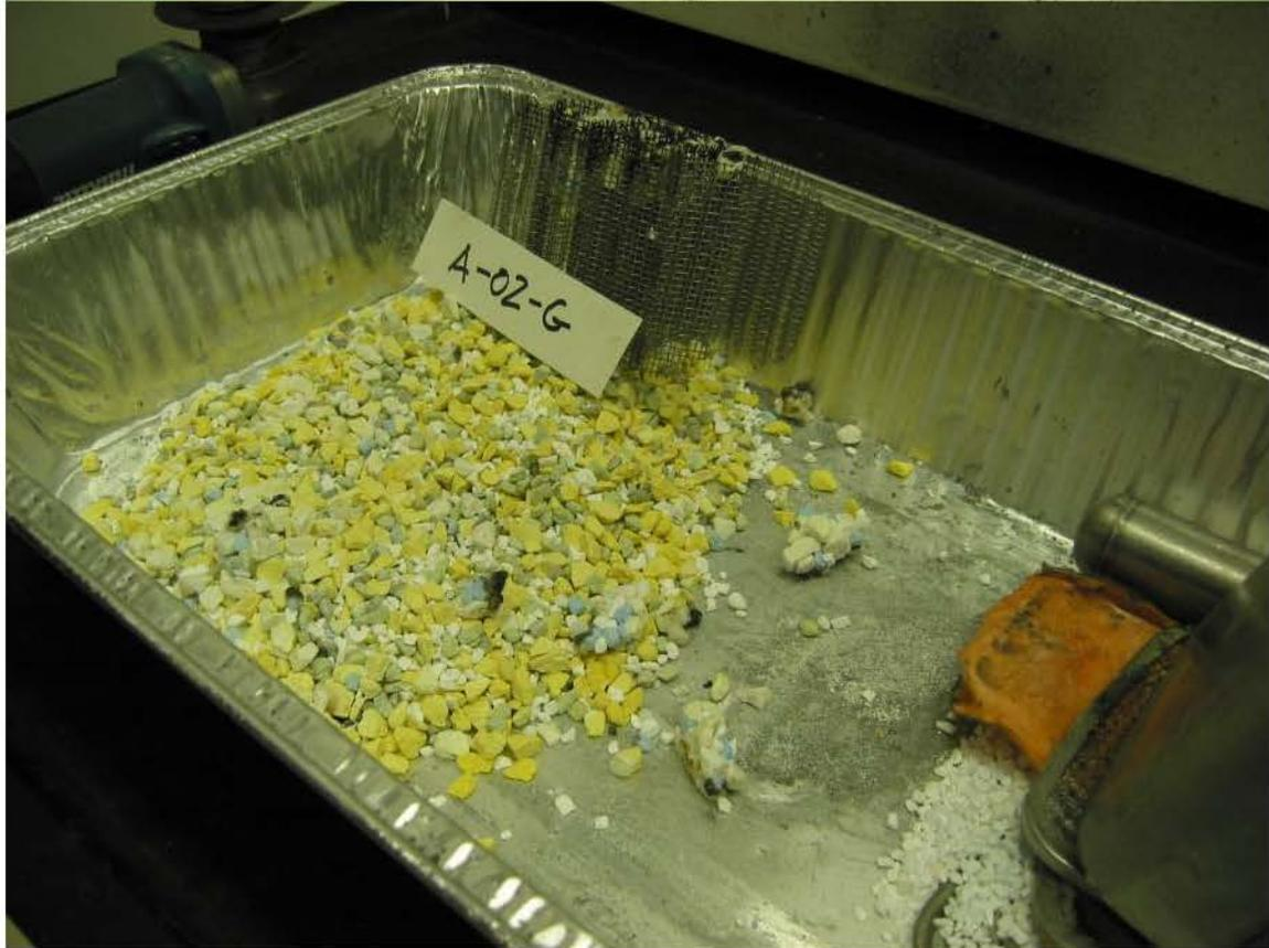
Figure 12 - Unit A-02-G, as Received and Remaining Chemical
