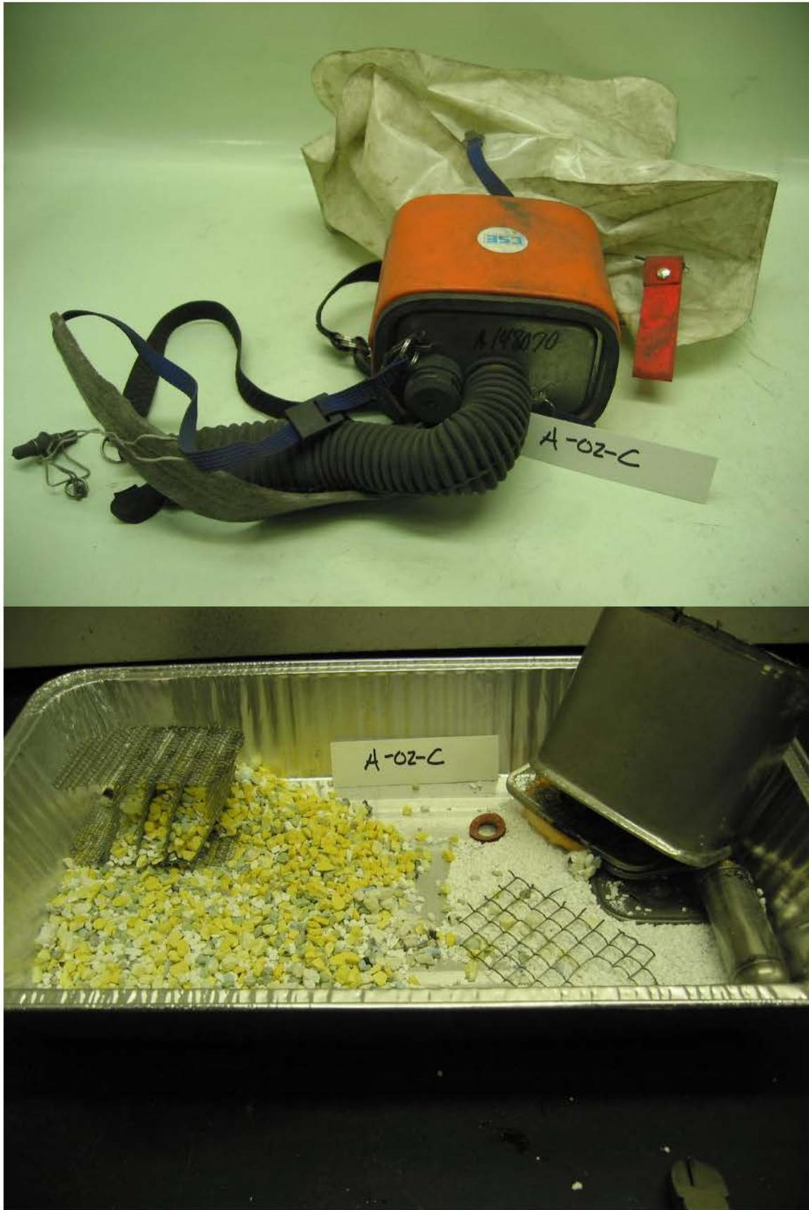
Figure 8 - Unit A-02-C, as Received and Remaining Chemical
