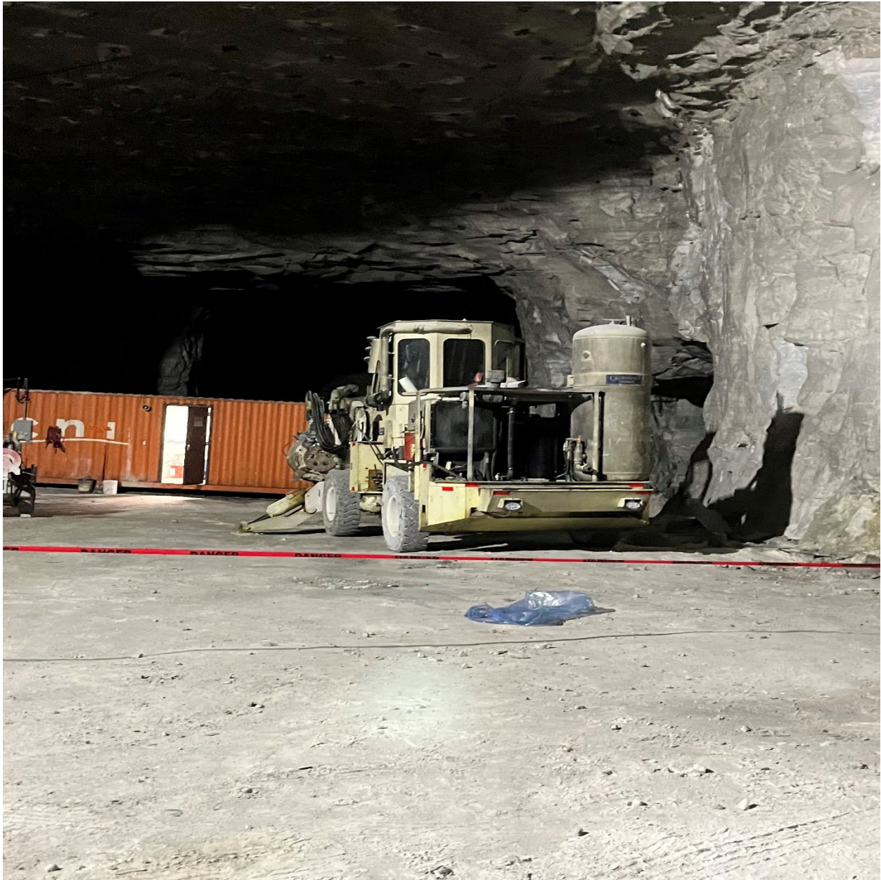
Photograph of the rear of the roof bolting machine, parked in the 740-parking area.
