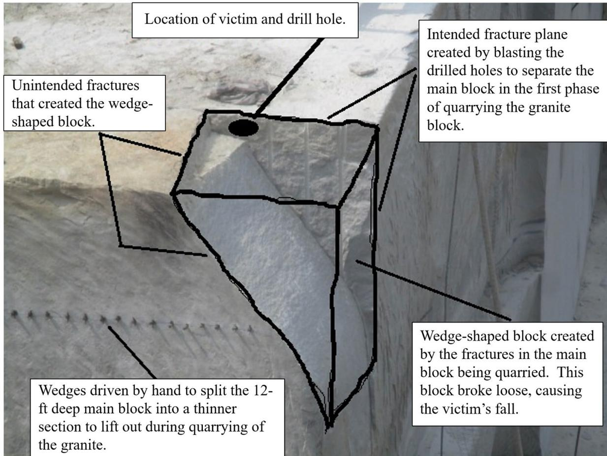
Zavala's location as he was drilling on the surface of the block in the wedge that was created by the crack. Annotations in the photograph indicate the drill hole location was within six feet of an edge where a fall would be significant.
