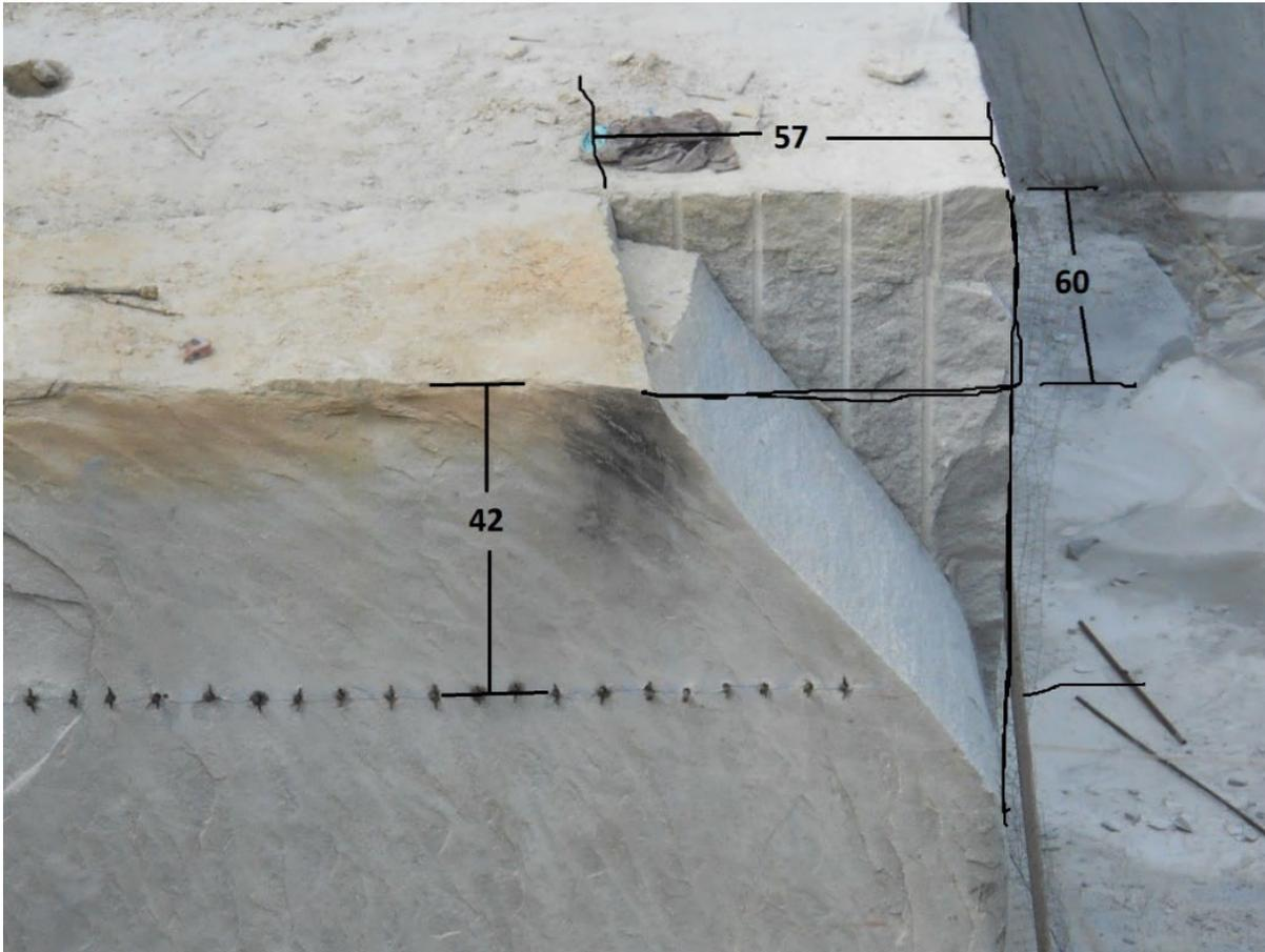
Dimensions, shown in inches, of the wedge-shaped block that broke and fell, causing Zavala to fall.
