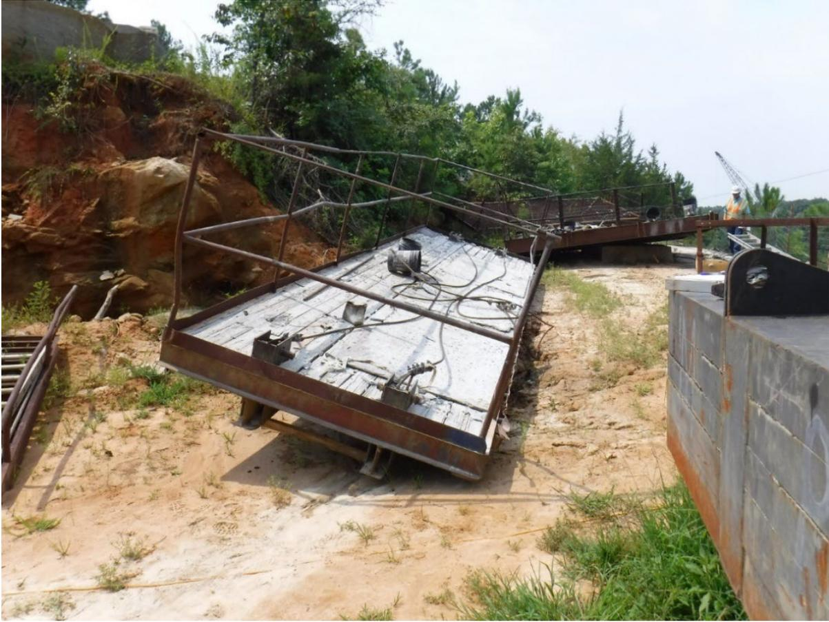
This scaffold was used to access the working face of the mining bench. A crane suspends the scaffold along the face of the mining bench.
