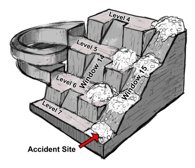
\*Note: This drawing is only meant to illustrate what the term "Windows" are used at the Kimballton Plant #1's Mine and do not reflect the mine's actual layout.
