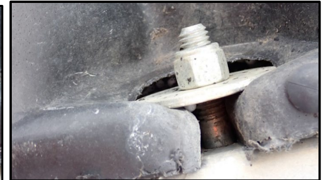
Float 2 – Plastic shell cracked at the front inner and rear inner bolt locations.
