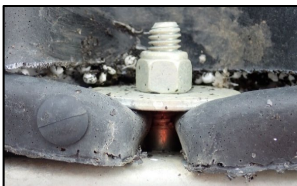
Float 2 – Plastic shell cracked at the front inner and rear inner bolt locations.
