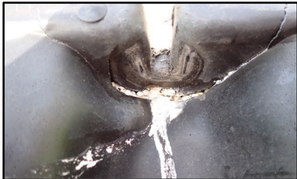
Float 1 – Plastic shell cracked at the front outer and rear outer bolt locations.
