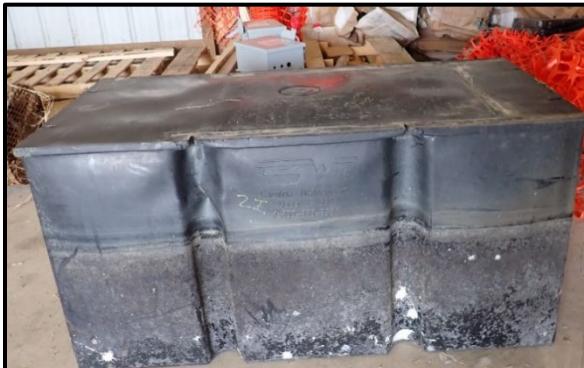
Float 2 – Plastic shell sidewall buckled at rear inner and Float 3 – Plastic shell cracked at rear outer bolt locations.
