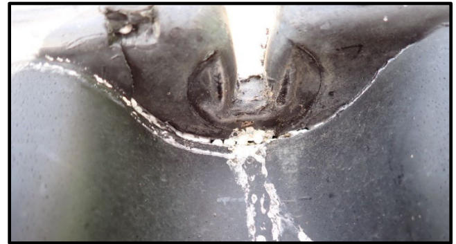
Float 1 – Plastic shell cracked at the front outer and rear outer bolt locations.
