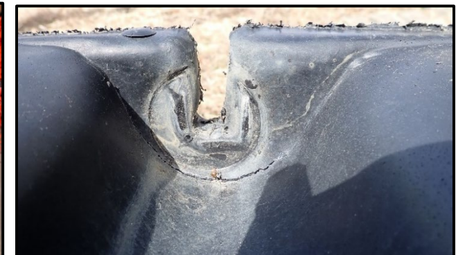
Float 2 – Plastic shell sidewall buckled at rear inner and Float 3 – Plastic shell cracked at rear outer bolt locations.
