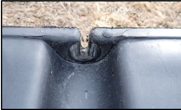
Float 1 – Plastic shell cracked at the rear inner and front inner bolt locations.
