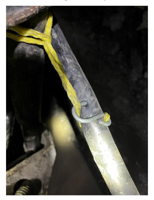
APPENDIX C – Trailing Cable Punctured by Metal S-Hook
