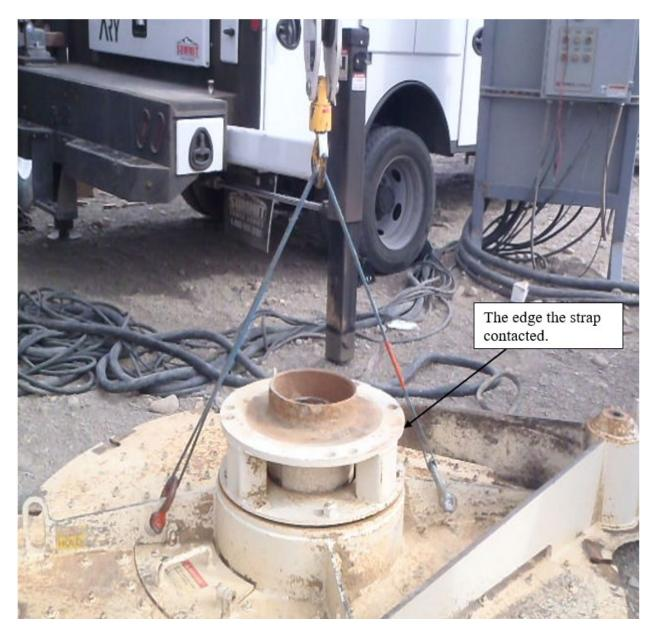
APPENDIX A – Nylon Lifting Strap Attached to the Lid
