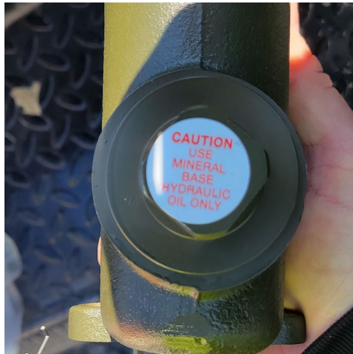
Figure 2: Brake Master Cylinder designed for Stryker service brake system
