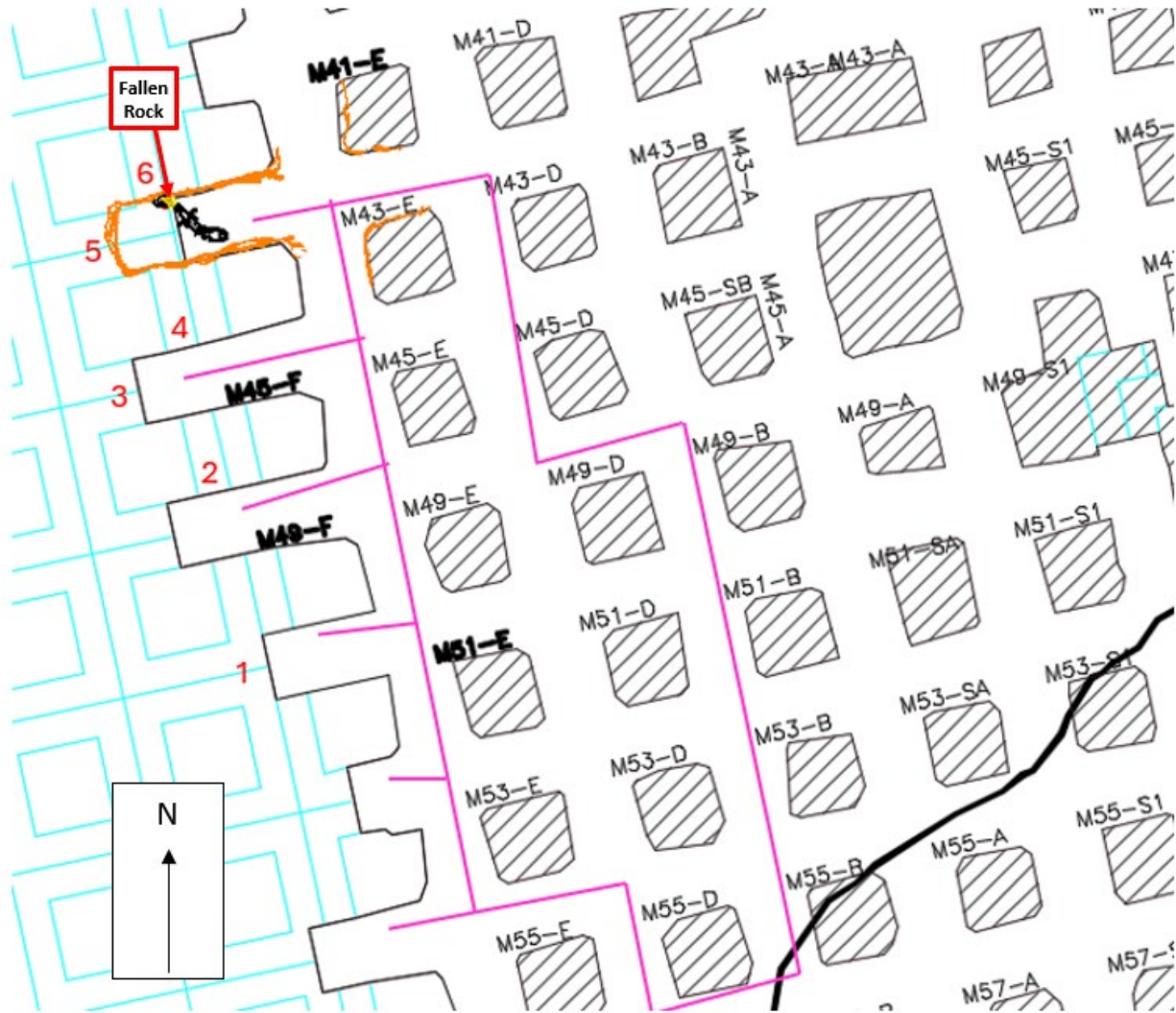
General map of showing observation traverse in magenta. Projected pillars are shown in cyan. Accident heading, as mined when the accident occurred, outlined in orange with the personnel lift shown in black and fallen material shown in yellow. The loaded faces are numbered in red.
