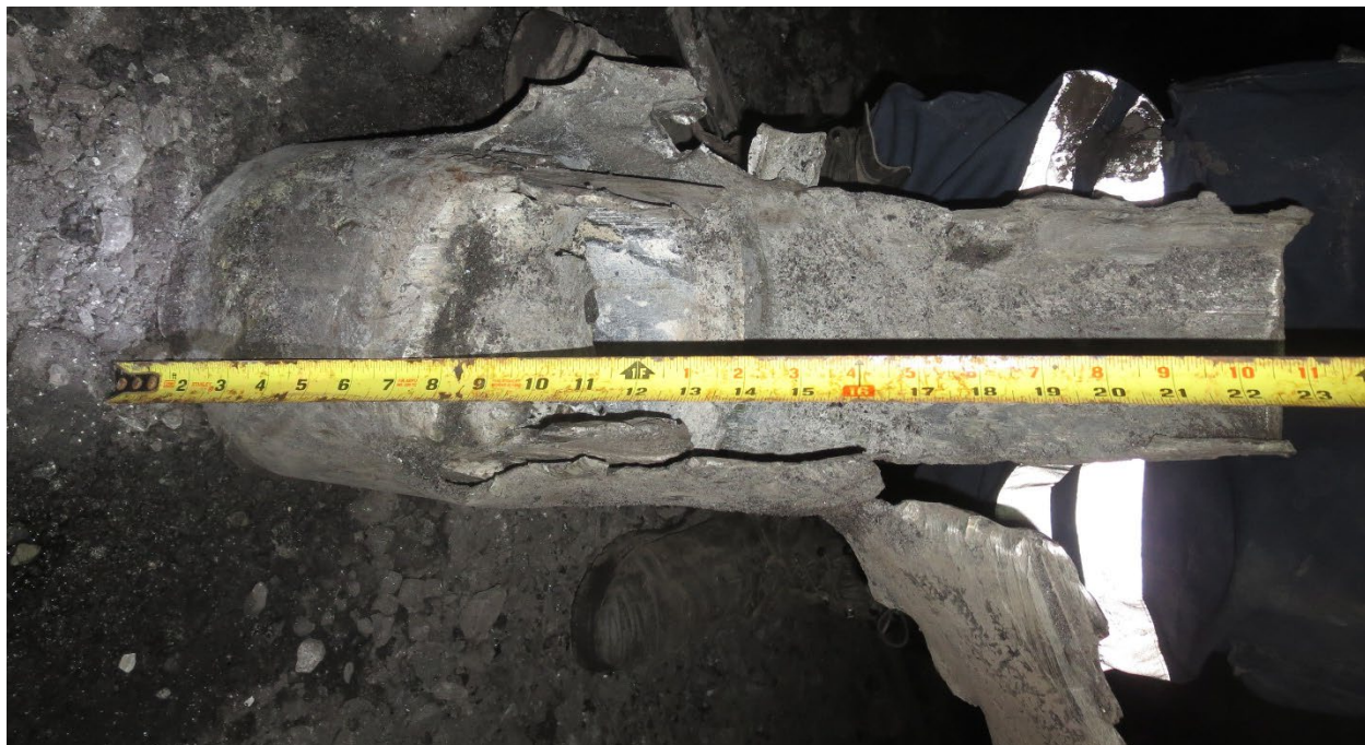
FIGURE 9.—A portion of well structure recovered after cut-through.
