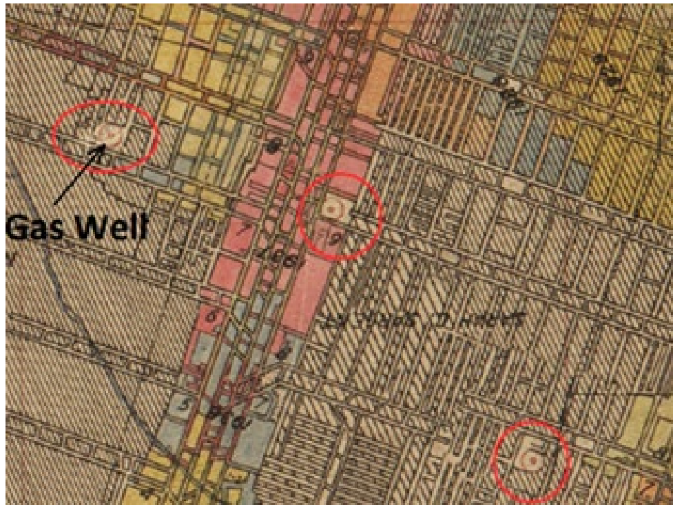
FIGURE 1.—A portion of a mine map from southwestern Pennsylvania during the hand-loading era, showing three gas well protective pillars surrounded by pillar recovery.
