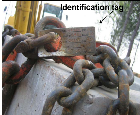
Unrated chain, clevis grab hooks and broken link
