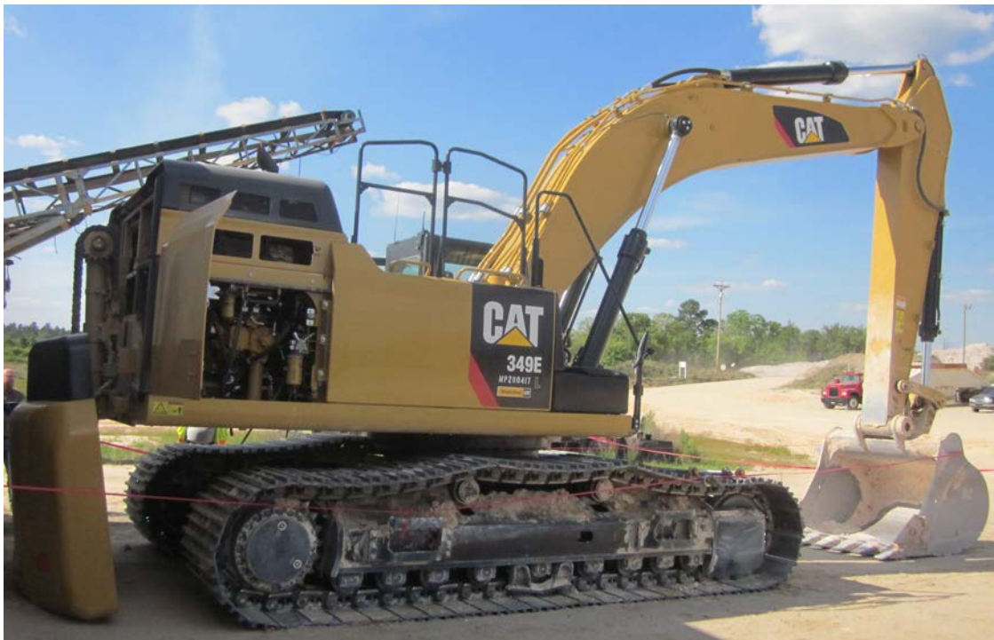
Illustration 1: Side View of Excavator showing dropped counterweight
