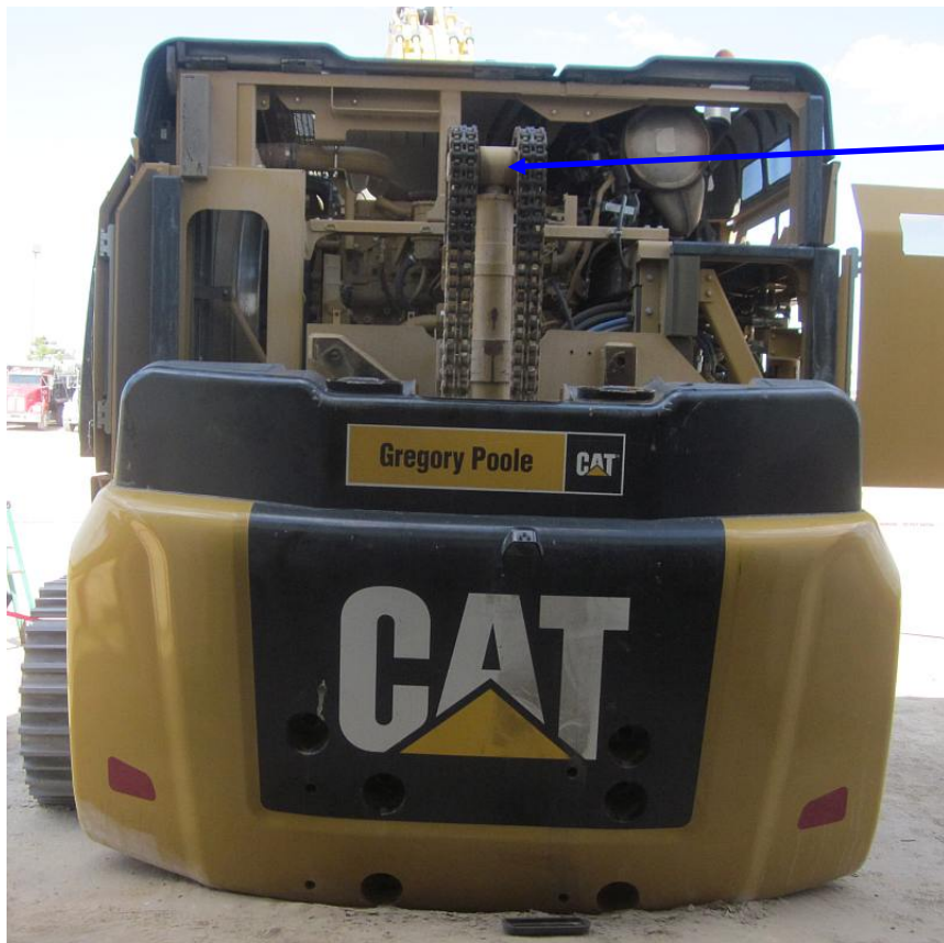
Illustration 2: Rear View of Excavator showing dropped counterweight
