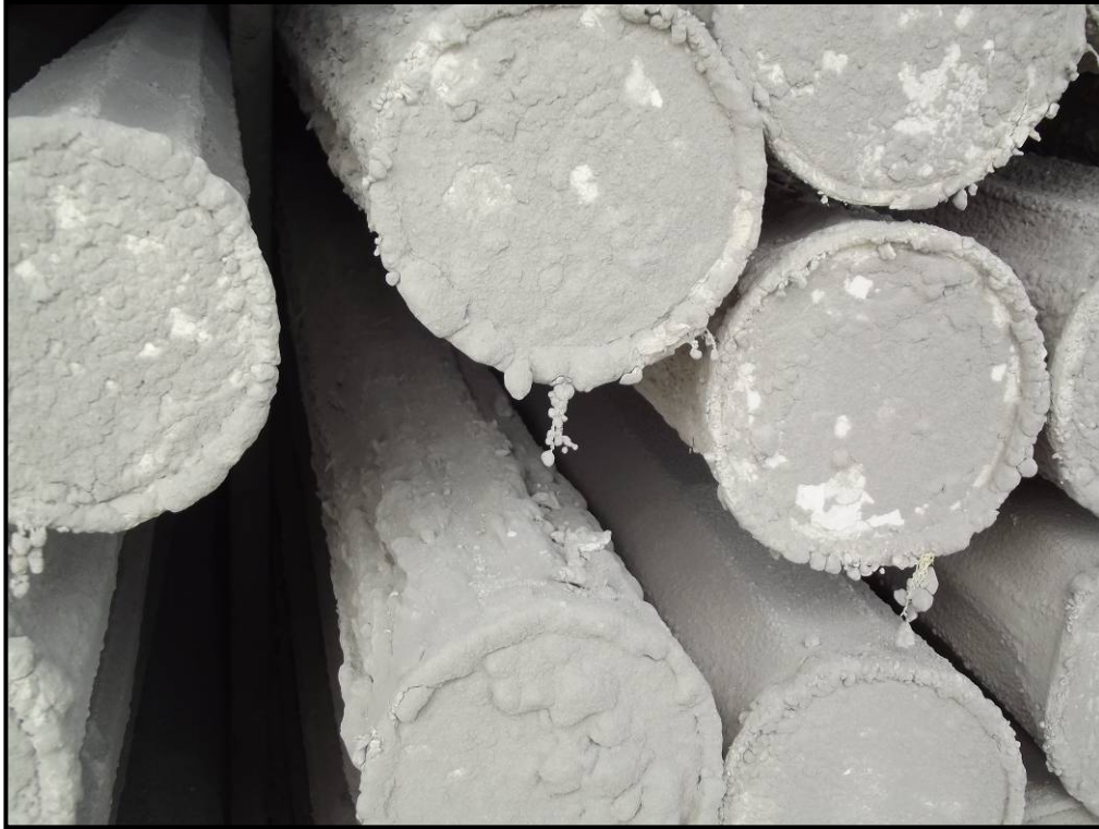
Photo 7 – Air filter bags in the Silo 12 dust collector were partly caked.
