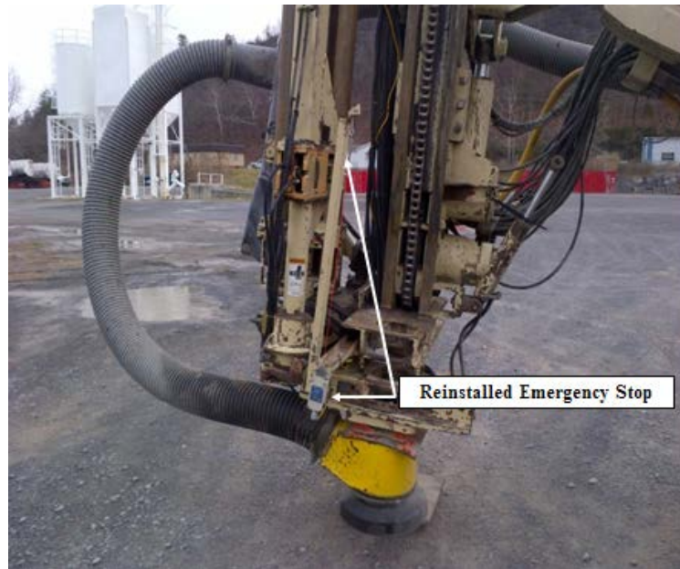
Figure 4 – Photo of Drill (Post-Accident)
